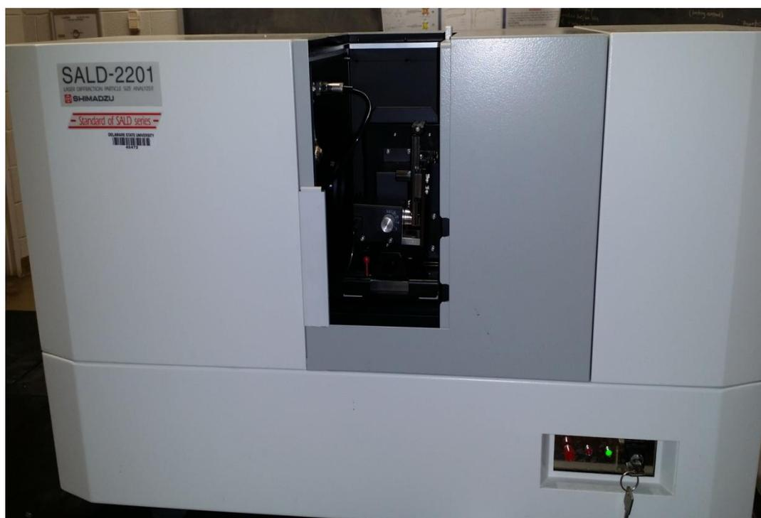
***Fig. 2.5 Laser diffraction particle size analyzer (Model: SALD-2201) from Shimadzu. Courtesy of Delaware State University, Dover. Center for Hydrogen Storage and Research (CHSR)***
