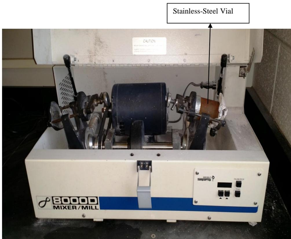
**Fig. 2.1** Ball-milling machine, courtesy of Center for Hydrogen Storage and Research (CHSR) laboratory at Delaware State University, Dover. U.S.A.
