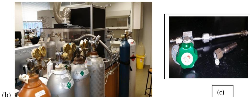
**Fig.2.9. (a) Front-view of the Micromeritics HPVA 100 (VTI) volumetric analyzer.(b) Rare-view of the instrument showing all the different gas tanks connected. The insert photo shows the sample holder (2cc) with the gasket supplied by Swagelok. Courtesy of Delaware State University, Dover. Center for Hydrogen Storage and Research (CHSR)**
