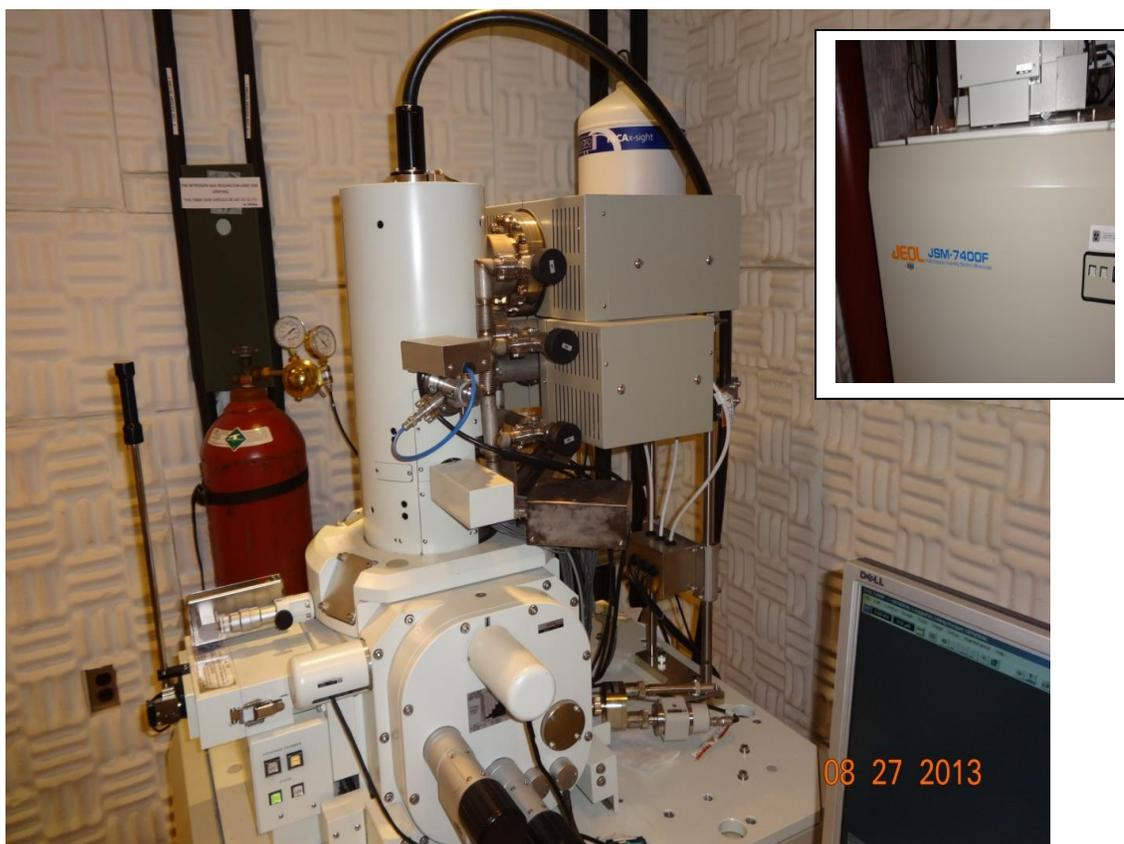
***Fig. 2.11. JOEL JSM 7400F scanning electron microscope instrument, with insert snapshot of its resting base. Courtesy of University of Delaware, U.S.A. Center for Material Sciences, Department of Chemistry***
