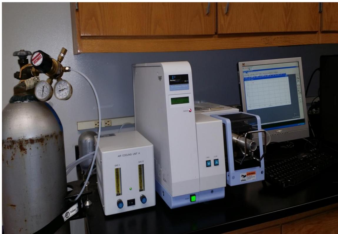
***Fig. 2.4. The Perkin-Elmer Diamond TG/DTA Analyzer. Courtesy of Delaware State University, Dover. Center for Hydrogen Storage and Research (CHSR)***
