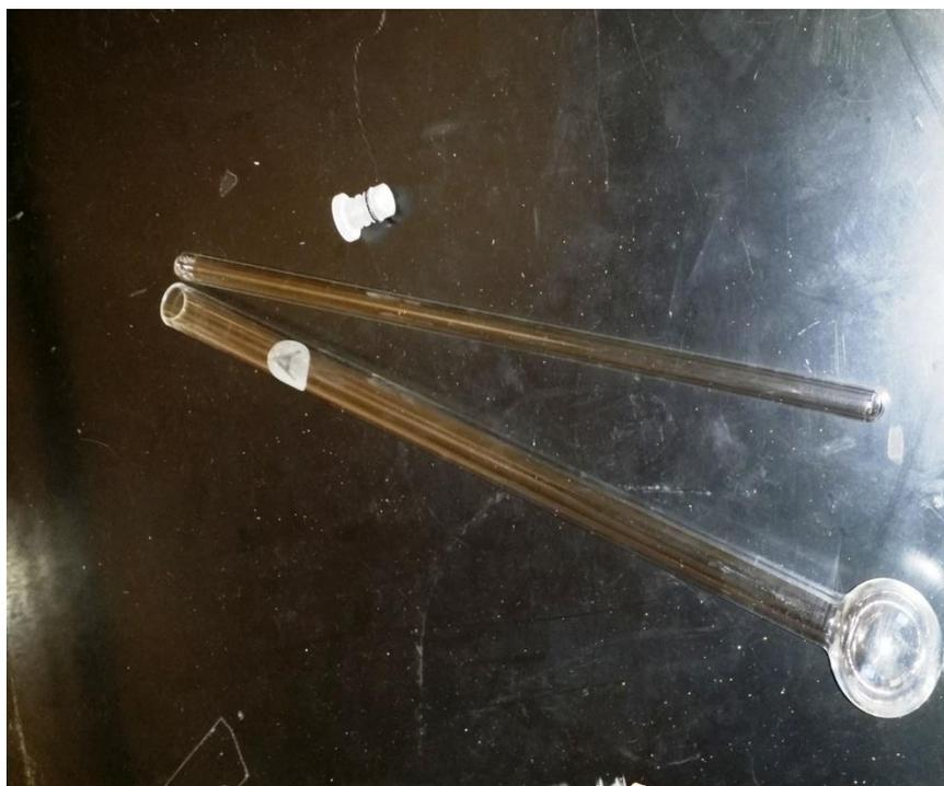
***Fig. 2.8. Sample glass-tube, filler rod and seal frit used for BET and gas adsorption analysis. Courtesy of Delaware State University, Dover. Center for Hydrogen Storage and Research (CHSR)***
